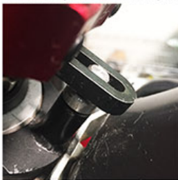
Correct! Top Is Flush With Top of Damper Arm.
