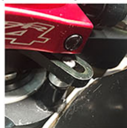
Enough Clearance For The Damper And Free Movement
